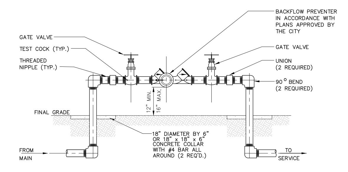
1. ALL PIPE AND FITTINGS 2" AND SMALLER SHALL BE THREADED SCHEDULE 40 GALVANIZED STEEL OR BRASS.
