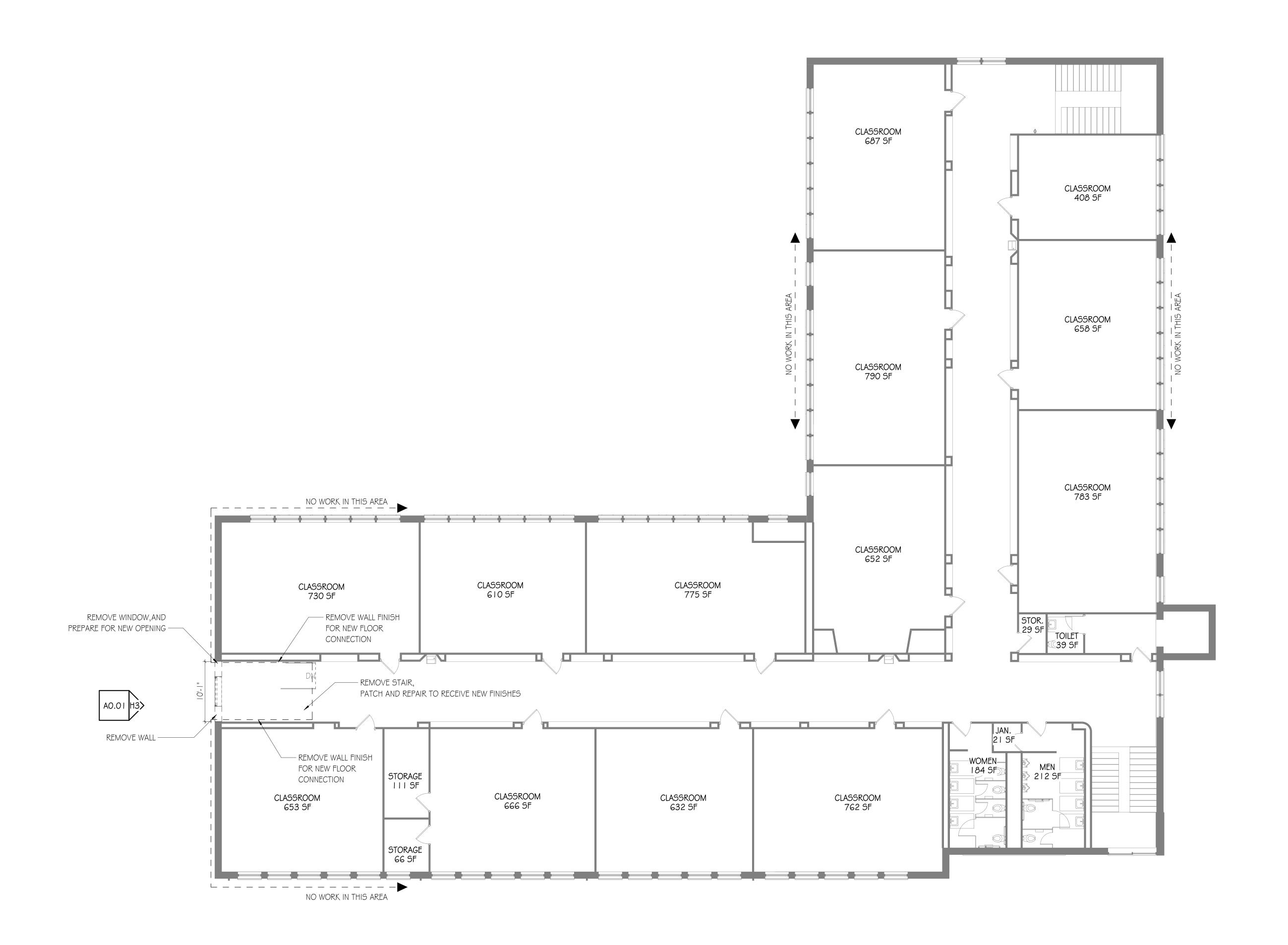
SECOND FLOOR DEMOLITION PLAN SCALE: 1/8" = 1'-0"
