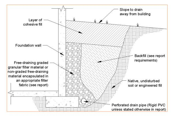
As an alternative to free-draining granular fill, a pre-fabricated drainage structure may be used. A pre-fabricated drainage structure is a plastic drainage core or mesh which is covered with filter fabric to prevent soil intrusion, and is fastened to the wall prior to placing backfill.
