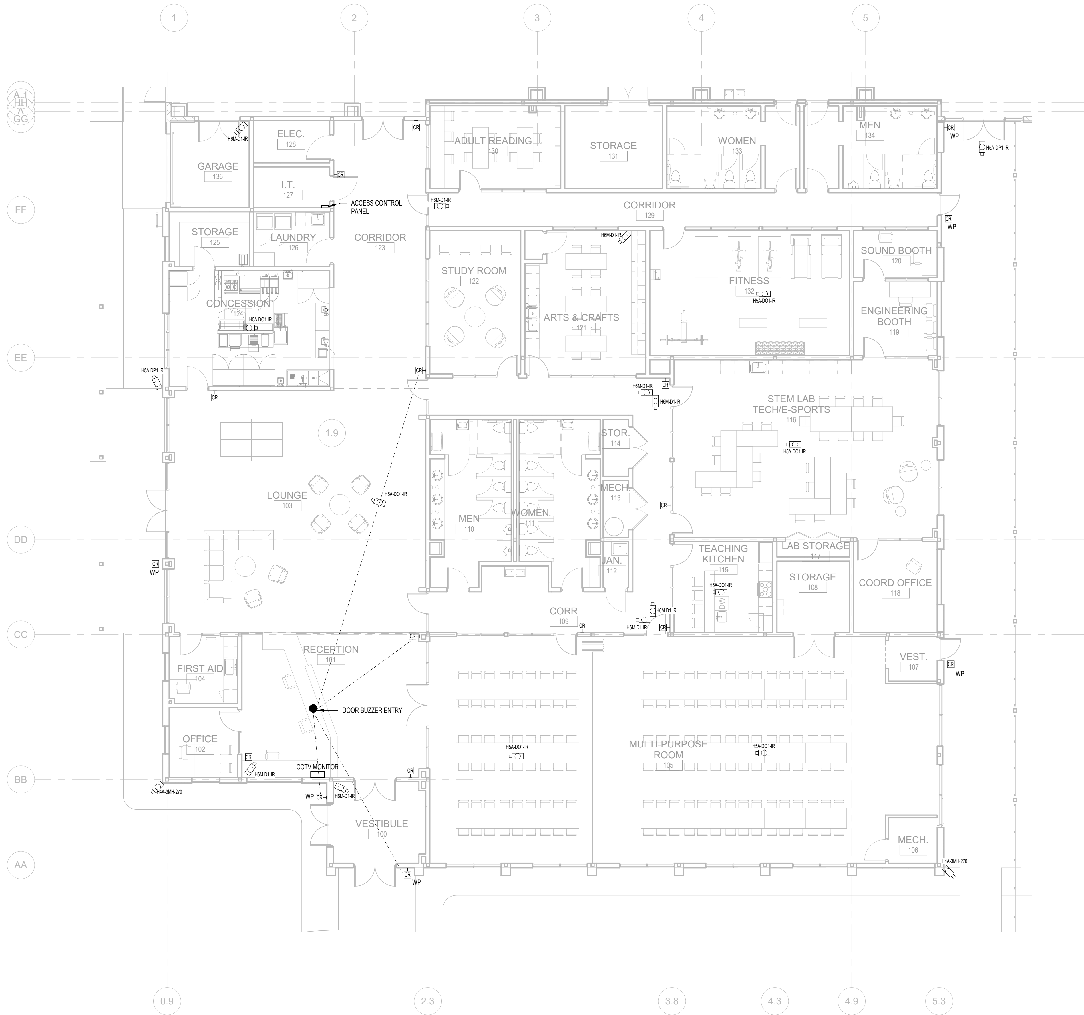
PROJECT NORTH 1 LV101 1/8" = 1'-0" 0 2' 4' 8' 16' LOW VOLTAGE - ZONE A
