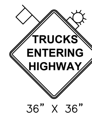
TRUCKS ENTERING HIGHWAY SIGN N.T.S.
