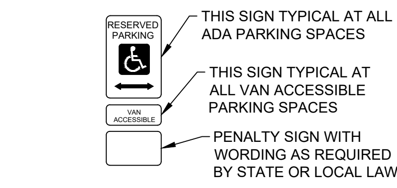
ADA SIGNAGE WALL MOUNT NOT TO SCALE
