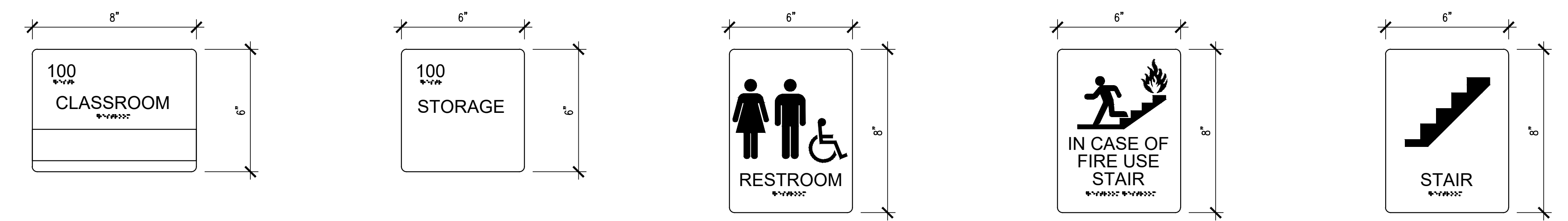
INTERIOR SIGNAGE (SIGN TYPE - A) SCALE: 3" = 1'-0" INTERIOR SIGNAGE (SIGN TYPE - B) SCALE: 3" = 1'-0" INTERIOR SIGNAGE (SIGN TYPE - C) SCALE: 3" = 1'-0" INTERIOR SIGNAGE (SIGN TYPE - D) SCALE: 3" = 1'-0" INTERIOR SIGNAGE (SIGN TYPE - E) SCALE: 3" = 1'-0"
