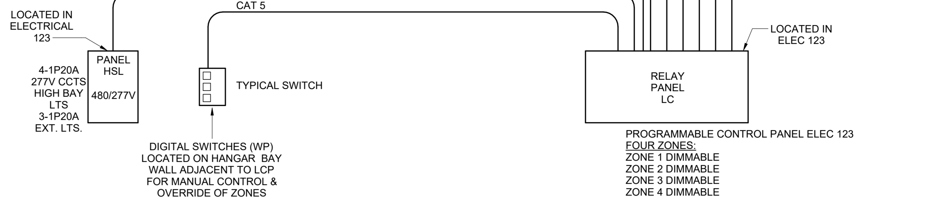
D3 HANGAR LIGHTING CONTROLS
