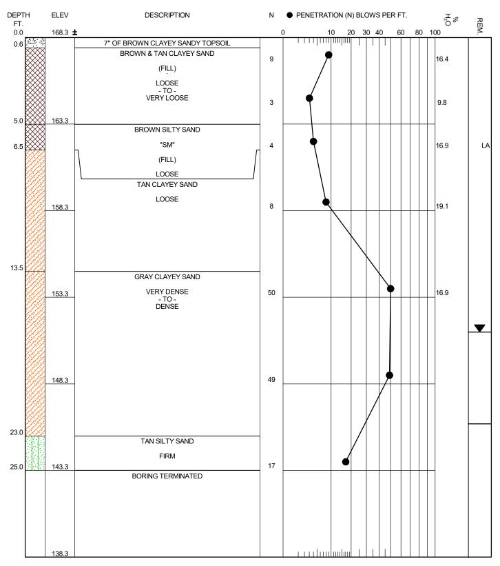
$\begin{array}{l} \mbox{Penetration (N) is the Number of Blows of 140 lb. Hammer \\ \mbox{Falling 30 in. Required to Drive 1.4 in I.D. Sampler 1 Ft. \end{array}$
