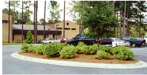
3-8g Landscaped islands improve the appearance of parking lots while providing shade and directing circulation.
