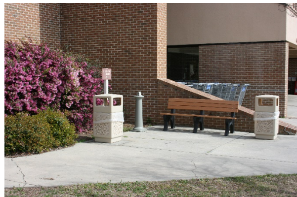
3-7f Trash can/ash receptacles at Commissary entrance constructed of precast exposed aggregate concrete with tan plastic tops.
