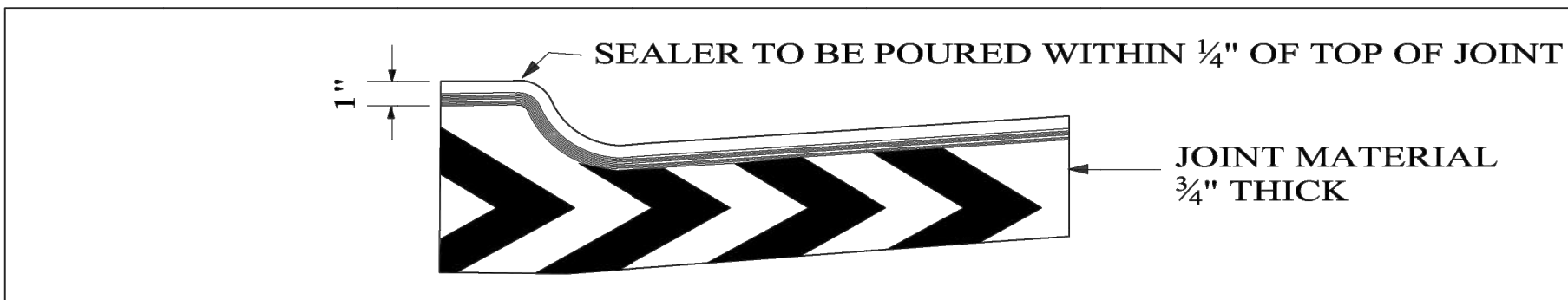
TYPICAL EXPANSION JOINT AND SEALER INSTALLATION
