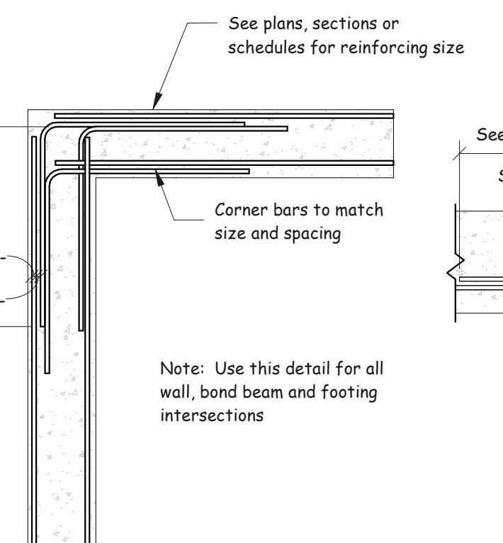
Typical Beam, Wall or Footing Reinforcing at Corners
