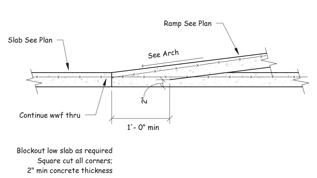
Slab on Grade Ramp Termination Detail
