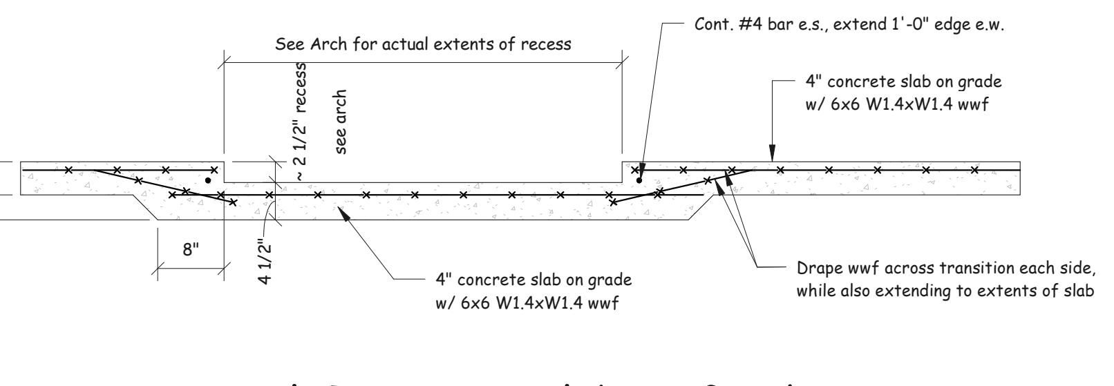
Typical Recess in Slab on Grade
