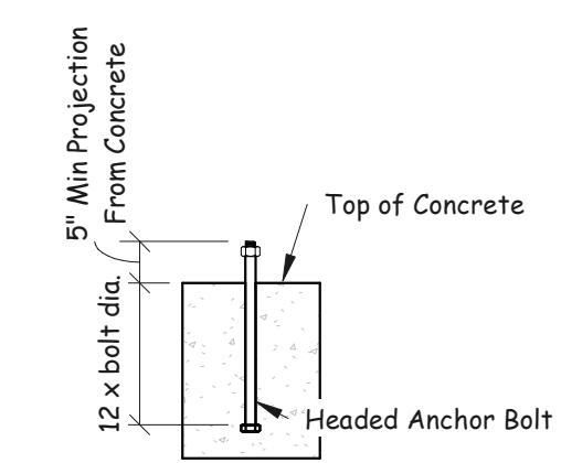
Typical Anchor Bolt Detail
